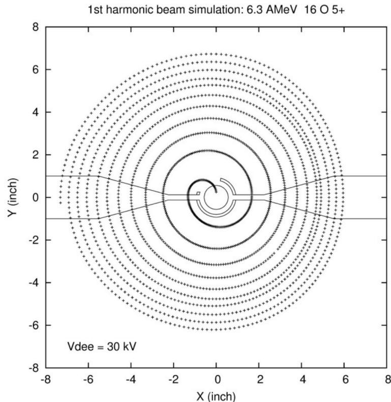
**FIG. 3.** First ten orbits of a 1st harmonic beam, specifically 6.3 AMeV  $^{16}\text{O}^{5+}$ , are shown. The beam exits from a mirror inflector at the center and into the dummy dee side before the acceleration begins.
