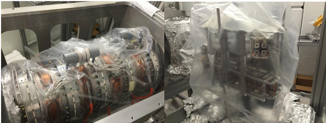
**FIG. 8.** Heavy ion guide gas catcher (left) and multi-RFQ (right).
